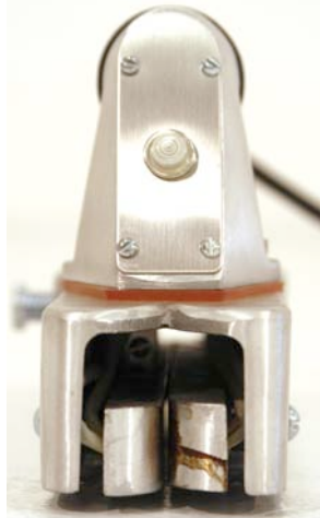
Pilot light indicates when temperature setting has been reached on pre-heater bars
