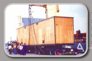
This 50 foot long international shipment loaded out of San Diego CA weighed in excess of 160,000 lbs. Inspection doors have been incorporated into the container sides at four points allowing additional anchor points for ship board tie downs to the actual machine.
